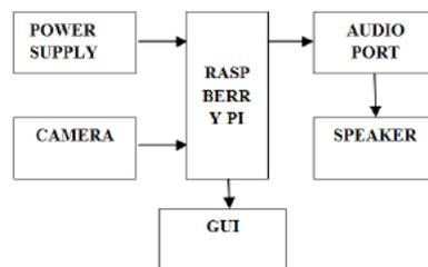
Fig. 1 Block diagram of TTS
