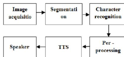
Fig. 2 Block diagram of OCR
