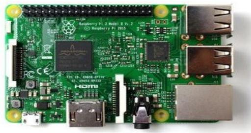
Fig -1: Raspberry Pi 3 Model B
